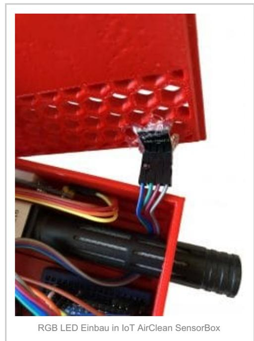
RGB LED Einbau in IoT AirClean SensorBox
